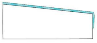
3mm Treadmaster should be turned over leading edge to provide vertical grip during horizontal thrust.
