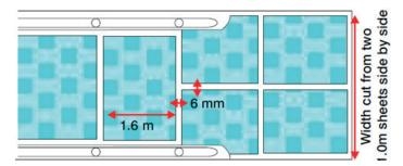
The 6 mm gap should be filled with a flexible mastic. (Sikaflex 11FC is recommended)
